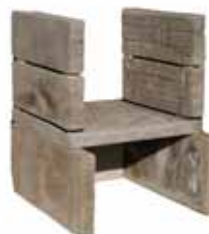
Step 9 - Add firebrick to walls
